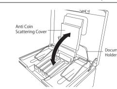
The "coin anti scattering cover" prevents the scattering of the coins inside the coin tray when carrying the cash box.
